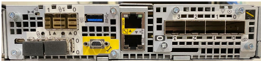
Figure 24. Embedded module with 4-port card
