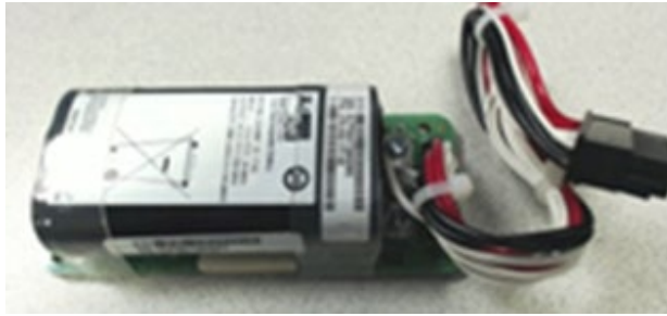
Figure 6. Battery backup unit
