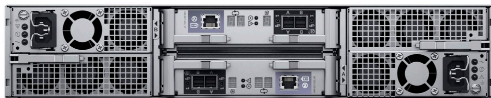
Figure 30. 25-drive 2.5-inch 2U expansion enclosure (back)
