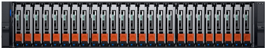
Figure 29. 25-drive 2.5-inch 2U expansion enclosure (front)
