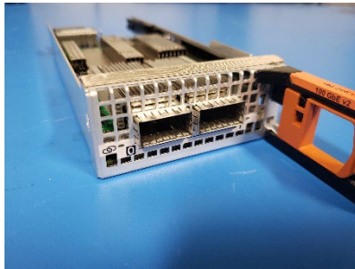
Figure 31. 100 GbE optical I/O module
