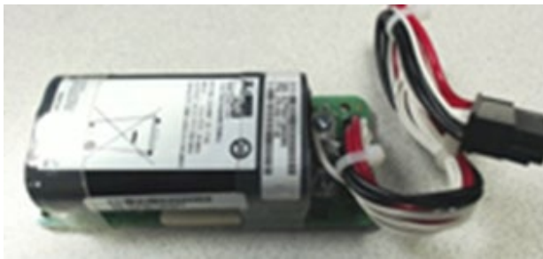
Figure 15. Battery backup unit
