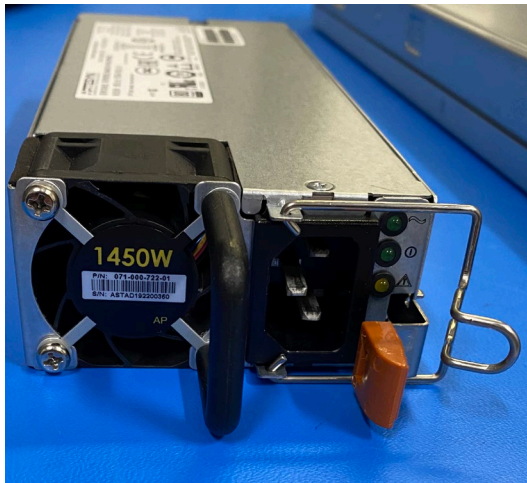
Figure 26. 1450 W power supply
