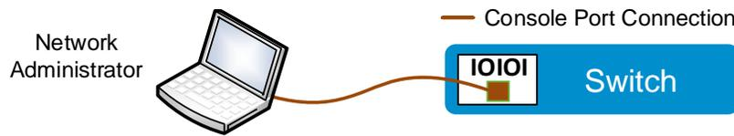
Figure 5 Connecting to a single device through the console port
