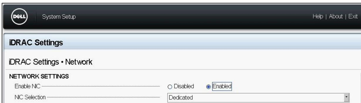
Figure 12 iDRAC NIC settings in System Setup
