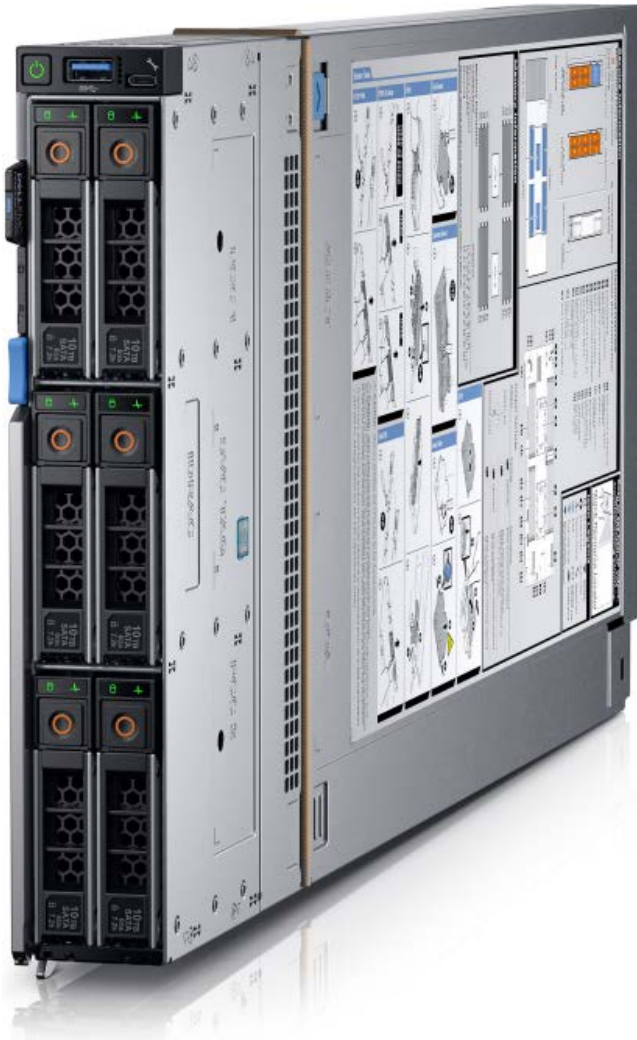
Figure 96 Dell EMC PowerEdge MX740c sled with six 2.5-inch SAS drives
