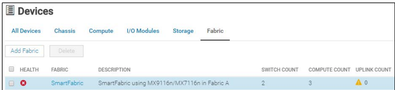
Figure 12 SmartFabric post-deployment without defined uplinks
