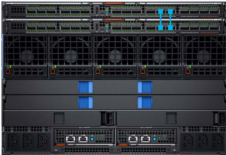
Figure 7 IOM placement – 2 x MX9116n in the same chassis
