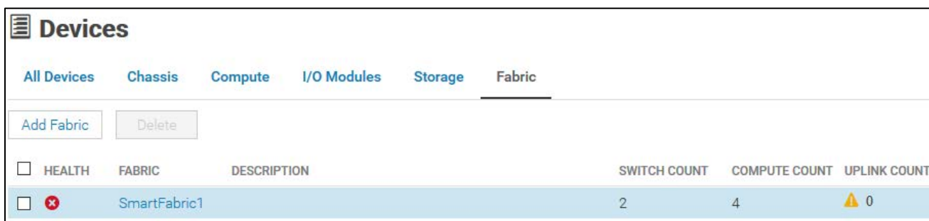
Figure 70 SmartFabric after deployment before uplinks are created
