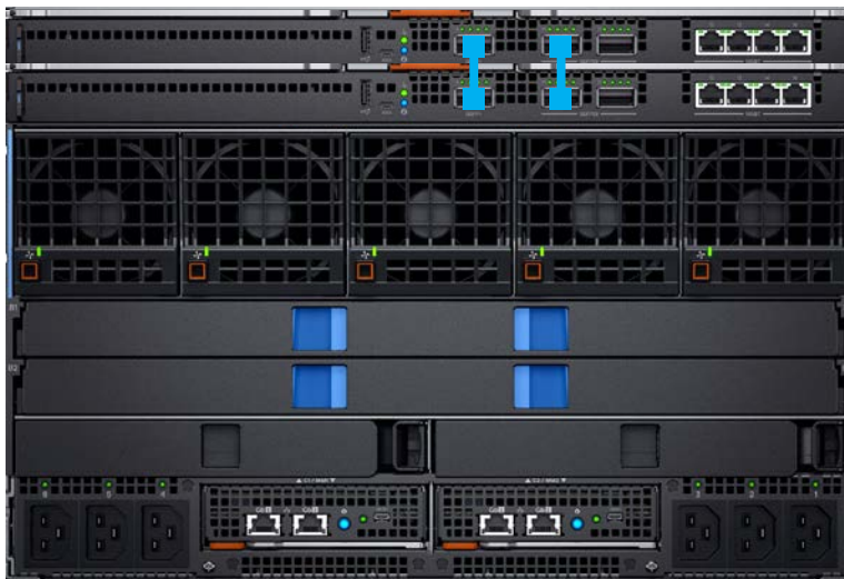
Figure 6 IOM placement – 2 x MX5108n in the same chassis
