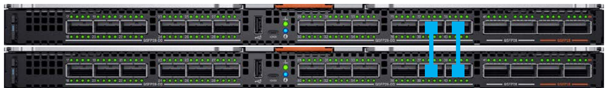
Figure 8 MX9116n SmartFabric VLTi cabling
